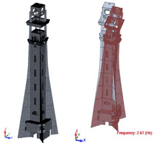
Figure 8. FEM modelling and modal analysis
