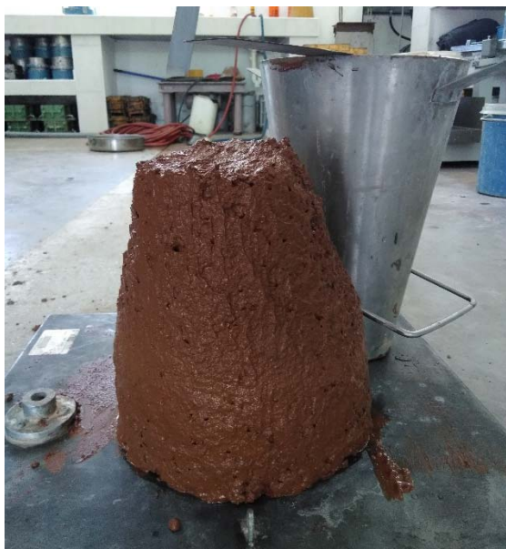
Figure 4. Mixture of concrete with high percentage of red mud (20%)
