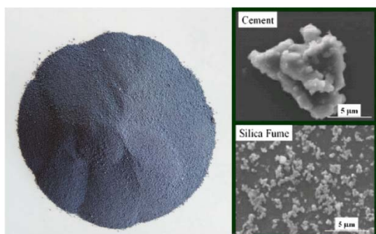
Figure 1. Silica fume in solid state (left) and comparison between cement and silica fume particle size (right)
