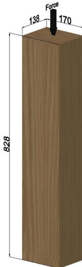
Figure 44. The example of application of load for the determination of compression strength parallel to the grain
