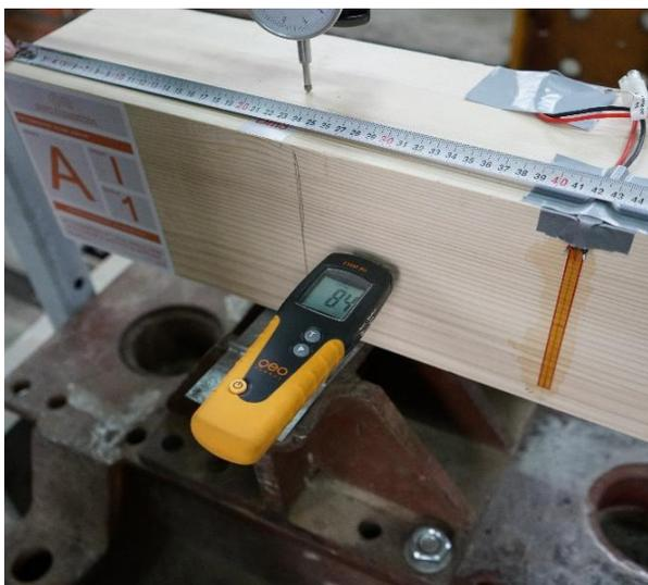
Figure 35. a) Measuring of Moisture Content
