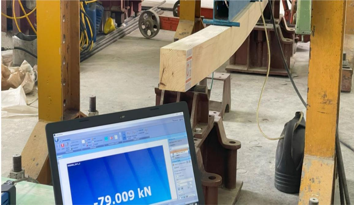
Figure 82. Experimental test for bending strength parallel to the grain
