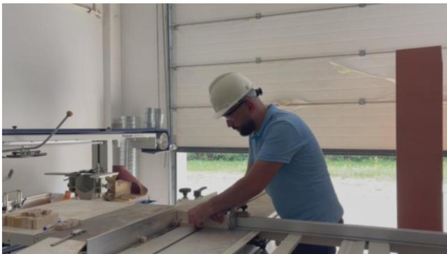
Figure 18. Cutting the test pieces according to EN 13183-1 on the designated sections
