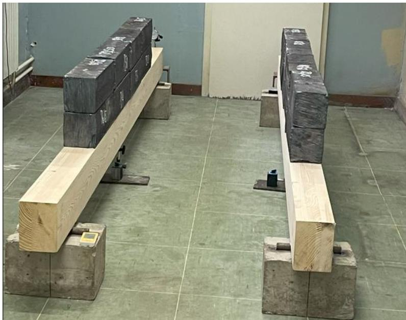
Figure 89. Long-term effect and creep coefficient under sustained load for DI1 and DI2
