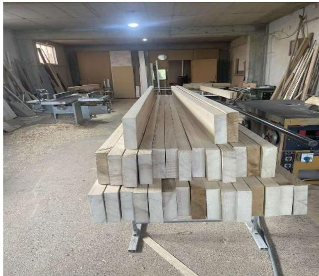
Figure 25. Selection and acquisition of the required lamellas
