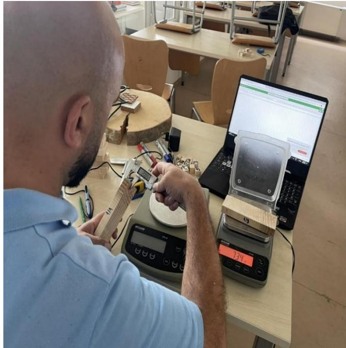
Figure 21. Measuring samples with caliper in three directions
