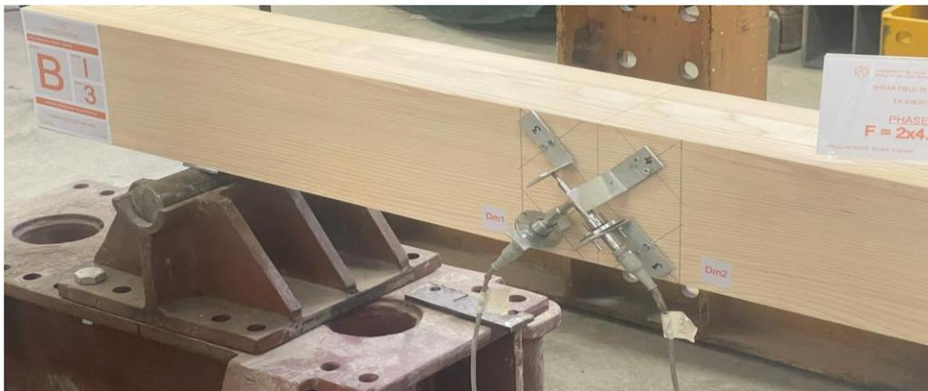
Figure 80. Shear-field experimental test accessories
