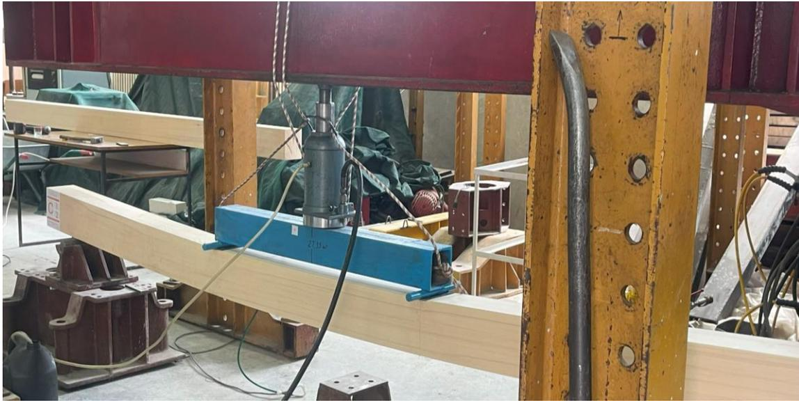
Figure 83. Experimental test for bending strength parallel to the grain
