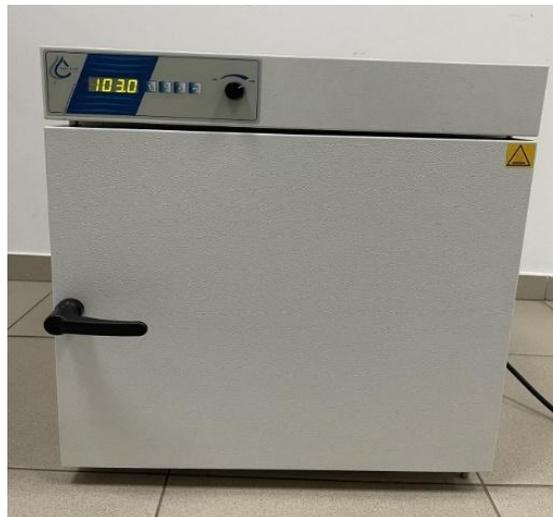
Figure 22. Adjustment of temperature in oven  $103 \pm 2^{\circ}\text{C}$
