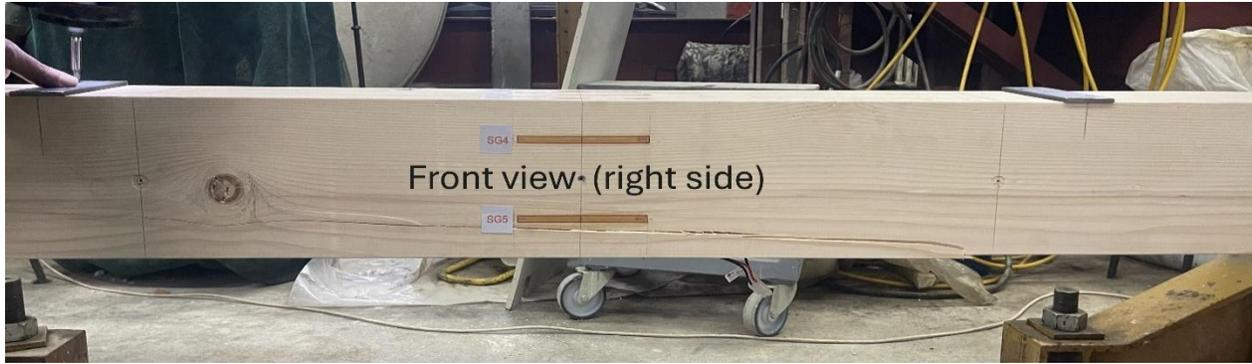
Figure 69. Front of the beam AI1 – defect and the crack description
