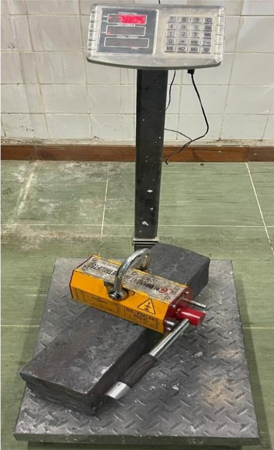
Figure 92. Weighing each of the steel billets
