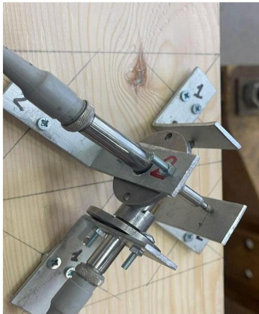
Figure 33. LVDT placement for shear field testing
