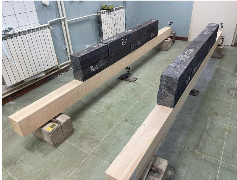
Figure 88. Determination of long-term behavior of beam DI1 and DI2
