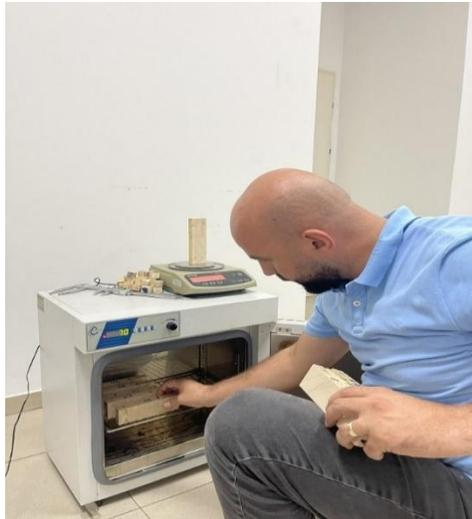
Figure 23. Placing the samples in the oven
