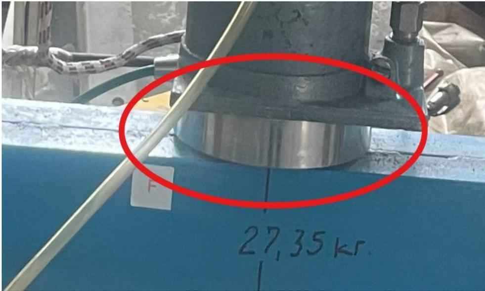
Figure 38. Load Cell, load applied through hydraulic jack
