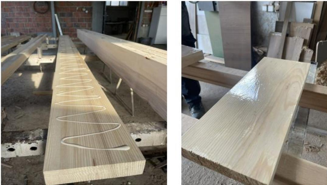
Figure 27. a) and b) Laying of glue with a thickness of more than 0.1 mm with the density of adhesive at around  $1,16 \text{ g/cm}^3$
