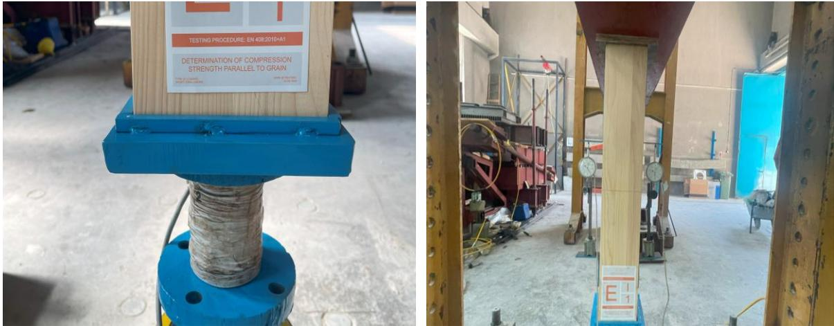
Figure 45. Experimental test of compression force parallel to the grain beam EI1
