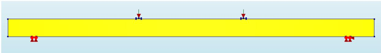
Figure 97. Arrangement of load application and support conditions in the numerical model
