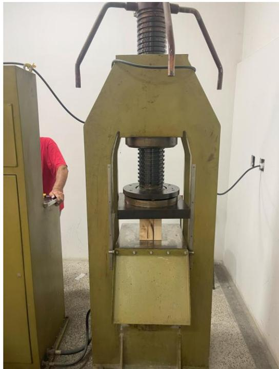
Figure 53. Press machine for determination of compression strength perpendicular to the grains
