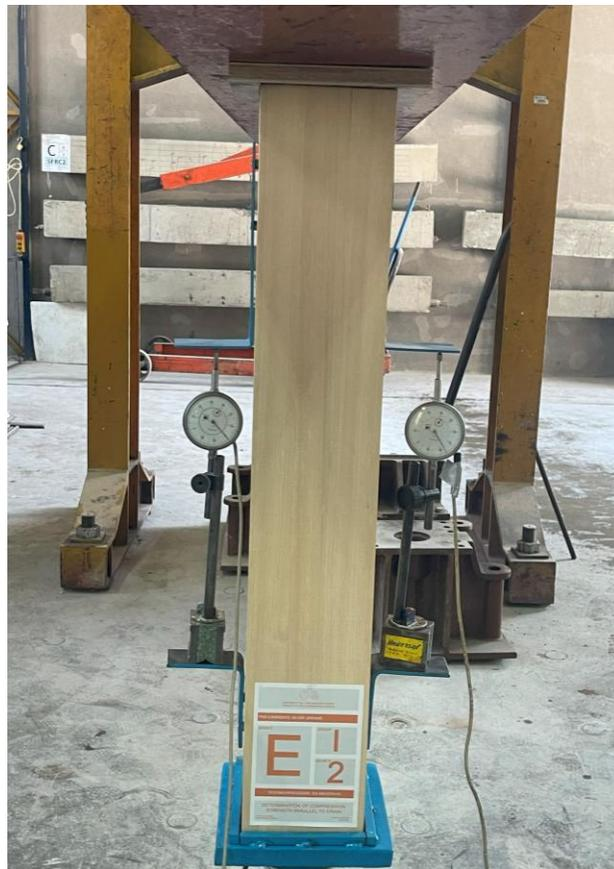
Figure 46. Experimental test of compression force parallel to the grain – beam EI2
