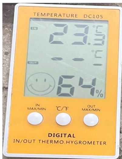
Figure 91. Equipment for temperature and relative humidity monitoring
