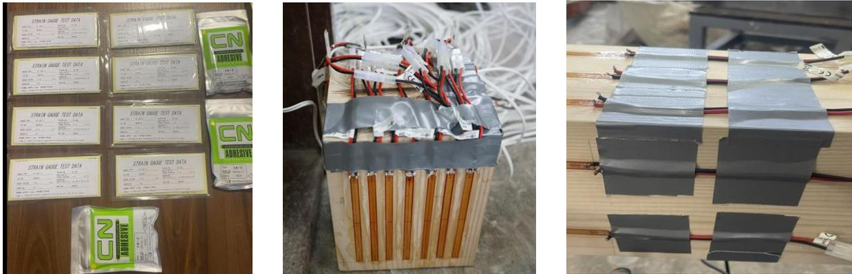
Figure 36. a) Strain gauges and special glue b) Strain gauges connection c) Strain gauges setting
