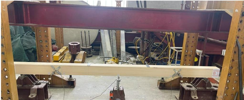
Figure 79. Experimental investigation of shear field test
